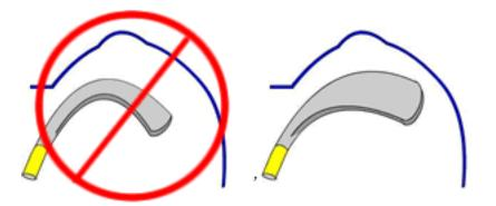
A spoon or dolly with a lower crown than the stretched area must be used when shrinking.
