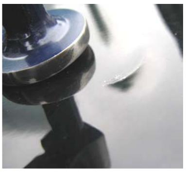
A slighty rounded hammer face edge and proper technique ensure cresent-shaped damage is not left by hammer blows.
