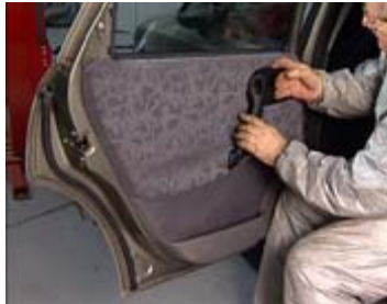
Replace the armrests and any other components, such as window winder mechanisms.
